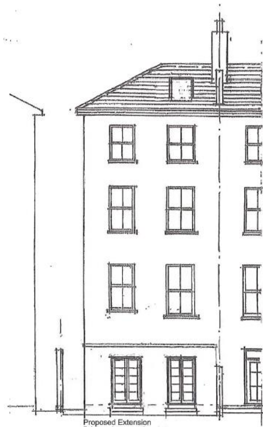
Proposed Extension Brickwork to match existing Traditional timber french doors Rear Elevation As Proposed.
